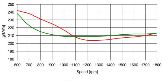
— full load curve — propeller curve
